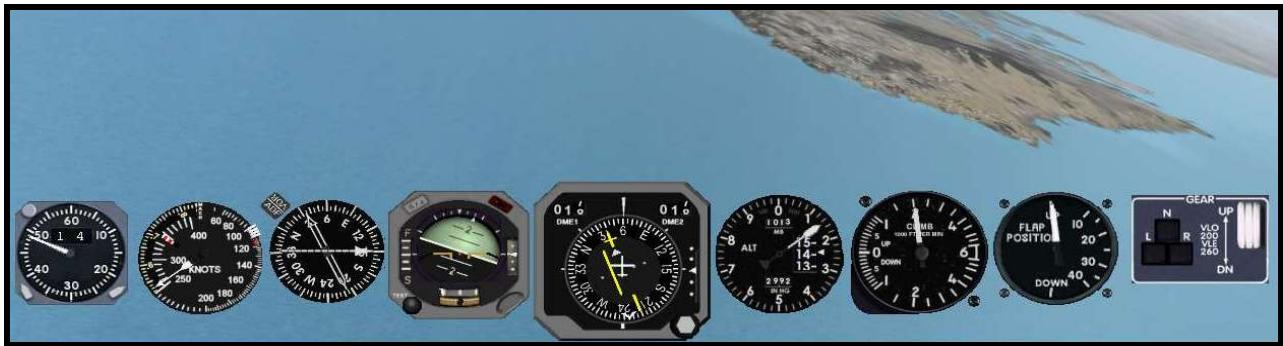
We are still in the turn, but as you can see with the RMI, it is pointing to about  $035^{\circ}$  to where the LAX VOR is located. We will level the wings when the RMI for the LAX VOR is pointing straight up and accelerate at that point.
