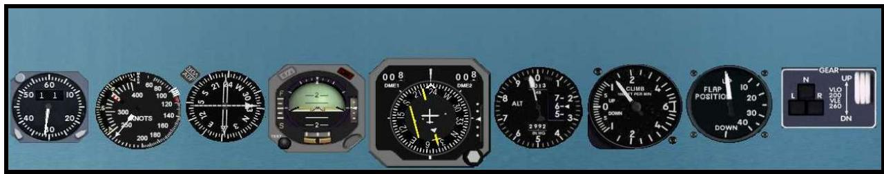
We have turned to a heading of  $235^{\circ}$  and are climbing out. Note that the DME is nearly 8 NM and that we are maintaining an indicated airspeed below 250 KIAS, since we are below 10,000' MSL.
