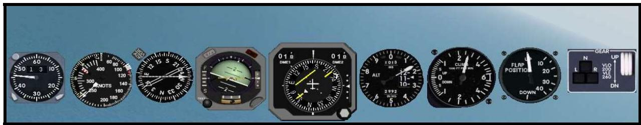
We are above 10,000' MSL and in the left turn. Note that we have not accelerated yet. We prefer to have a lower airspeed during the turn. Speeding up will only widen the turn, which is not desirable.
