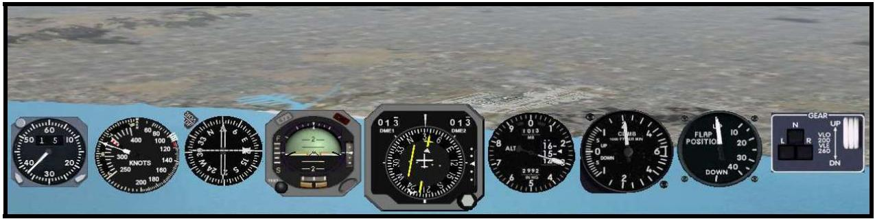
Here we see that the RMI is pointing straight ahead. We are now 13 NM from the VOR. Since we've completed the turn, we accelerate, and the DC-8 is very happy to comply. We simply fly this heading until the RMI needle turns around, indicating we are over the VOR.
