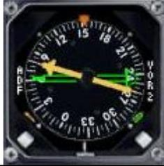
The ADF that we use on the DVA EMB-120 is built into the **RMI** (*Radio Magnetic Instrument*).
