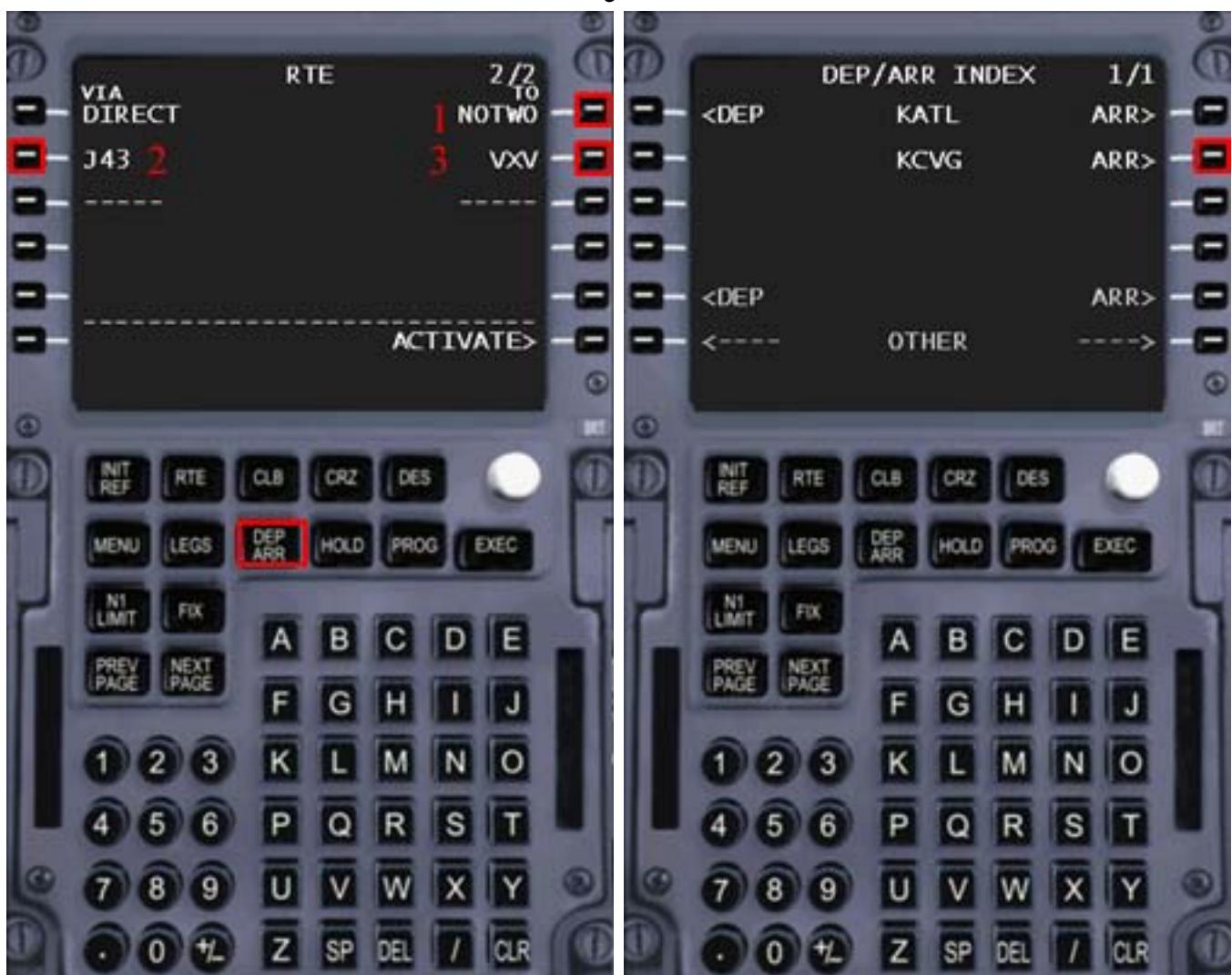
On this screen we will enter our route. We'll begin by entering NOTWO by using the input pad and then clicking the button next to the number 1 above. When you do this, DIRECT will show as the value for the button to the left. This is telling the FMC to fly direct to NOTWO from RWY 27R.
