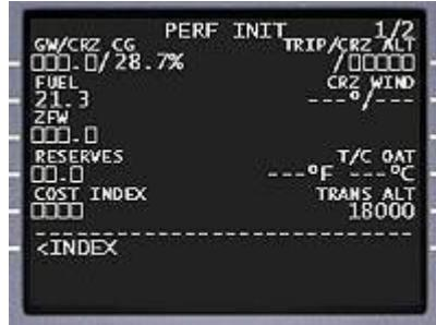
As with programming anything, there are certain data requirements that must be met. The FMC is no different. Whenever you see boxes as shown in the image above, it means that data is required there and must be inserted. Keep this in mind when programming the FMC for future flight.
